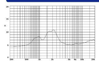
Note: on axis frequency response measured coupled to TD-164 horn in anechoic chamber, 2.83V @ 1m.
