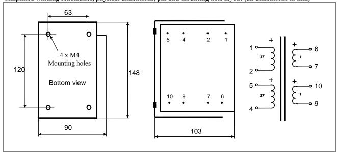
Weight: 4.6 kg $260 \Omega$ Static resistance of each primary:  $0.3 \Omega$ Static resistance of each secondary: 4 kV / 2 kV Isolation between windings / between windings and core: Max DC current through any primary winding (10W heat dissip): 140mA
